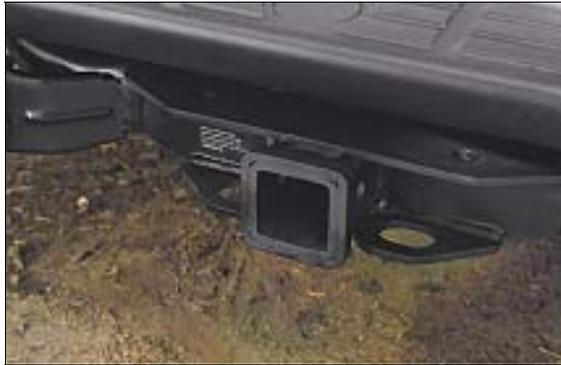
**Clamp-On Bumper Hitch** – As the name suggests, this type of temporary hitch clamps onto the bumper assembly. **Nissan does not recommend the use of this type hitch for a number of reasons.** It may interfere with performance of the energy-absorbing bumper. And because the bumper was not designed to carry this type of load, it could damage the bumper and bodywork, and may possibly result in trailer separation during towing. Therefore, **tow only with a permanent hitch.**
