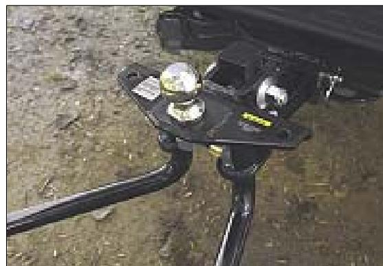
Purchase of a Weight-Distributing hitch ball mount (Class IV) is **STRONGLY RECOMMENDED** if you own an Armada or Titan vehicle and plan to tow trailers with maximum weight over 5,000 lbs. This ball mount includes a  $2\frac{5}{16}$ ” hitch ball rated for up to 10,000 lbs., and is available through your Nissan dealer for use with the optional tow package.
